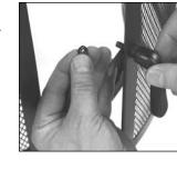
**6d.** Tighten the "jam nut" with a wrench.
